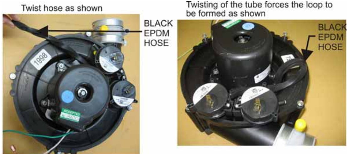
Figure 1: New routing of the EPDM hose in all single-stage furnaces as of 11/17/2008
