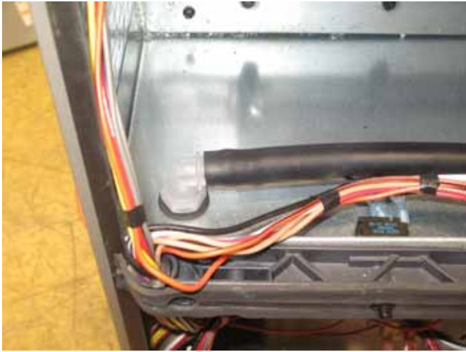
Figure 6 – Proper sealing for blower deck penetration
